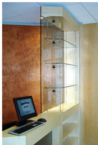
◀ Beech veneered reception counter with integrated illuminated display area featuring 4 x adjustable shaped glass shelves and low-voltage spotlights supported on satin chromed rods. O/A H1500 x W1100 x D350mm.
