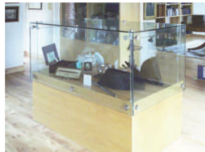
▲ Display case featuring 10mm glass secured to a light oak plinth using mirror polished stainless steel patch fittings. This cabinet also features 2 x 20 watt low-voltage adjustable spotlights suspended from bright chromed brass rods. O/A H1200 x W1300 x D600mm.
