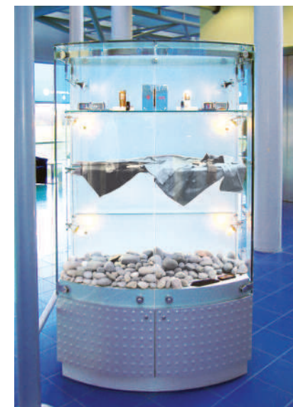
◀ ▶ Large display case consisting of a 10mm glass surround held with mirror polished stainless steel patch fittings to a white laminated plinth. Also featuring 4 x 20 watt low-voltage adjustable spotlights suspended from bright chromed brass rods. O/A H1850 x W1950 x D850mm.
