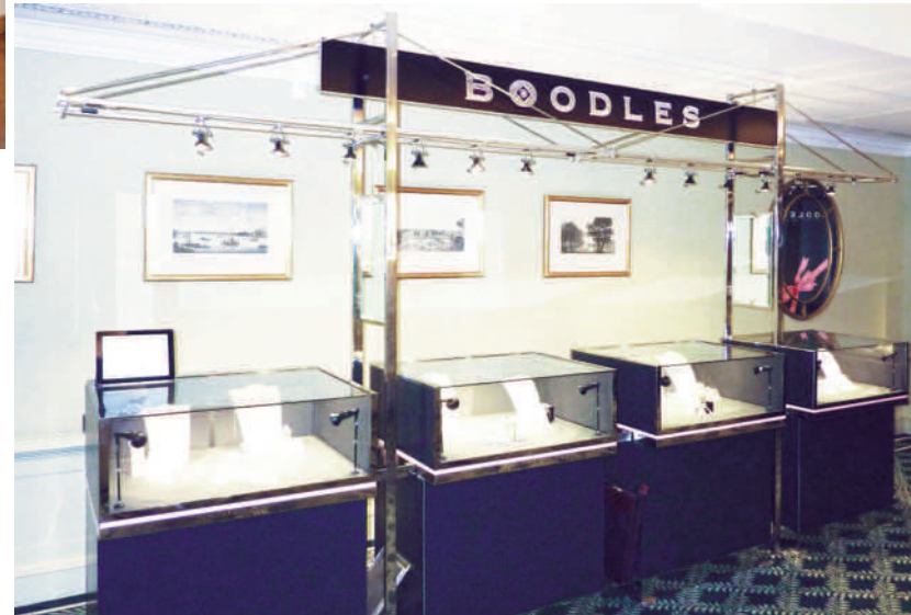
▲ Four illuminated glass jewellery counters produced in a durable dark charcoal laminate with mirror polished stainless steel kick-plate and trims. Each counter has a lockable pull out display area with lockable storage areas below and they are all connected together by the overhead gantry supporting signage and 12 x 50 watt low-voltage adjustable spotlights. Jewellery counters each O/A H100 x W800 x D500mm. Gantry O/A H2200 x W4200 x D300mm.
